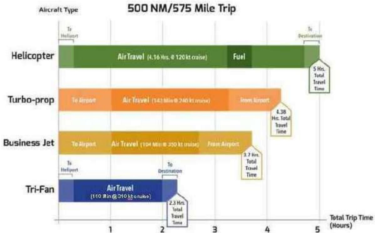
**Sample flight illustrating how TriFan 600 enables shorter trip times**
